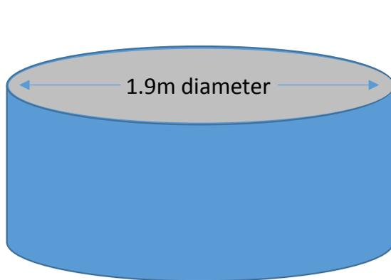
If installed in a circular pit, the diameter measures 1.9m when fully extended, but the membrane can easily be folded, to create smaller sizes, as required.
