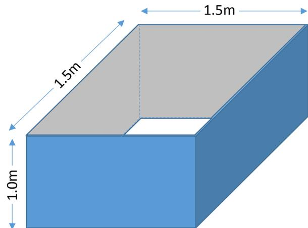
If installed in a square pit, the membrane will measure 1.5m on each of the four sides. Naturally, it can be folded to create smaller sizes, or installed in a rectangular pit.
