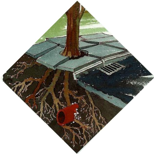
Installing **DENDRO-SCOTT™ Ready-Made Tree Pit Liners** is an excellent way to protect pavements, pathways, gardens, etc., from tree roots; diverting them downwards.
